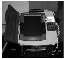
Figure 2. AccuVote TSx direct recording electronic device
